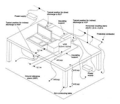
The test setup shall consist of a non-conductive table, (0.8±0.08)m high , standing on the ground reference plan.
