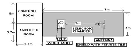
NOTE: The SPORTON 7m x 4m x 4m semichoic chamber is compliance with the sixteen points uniform field requirement as stated in IEC 61000-4-3 Section 6.2.
