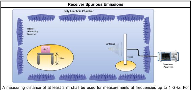
A measuring distance of at least 3 m shall be used for measurements at frequencies up to 1 GHz. For frequencies above 1 GHz, any suitable measuring far field distance may be used, depending on the test system noise floor for detecting spurious emission signals. The equipment size (excluding the antenna) shall be less than 20 % of the measuring distance. The height of the equipment or of the substitution antenna shall be 1.5 m.
